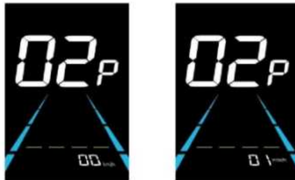
(02P is shown in the picture) Metric and Imperial unit setting interface
